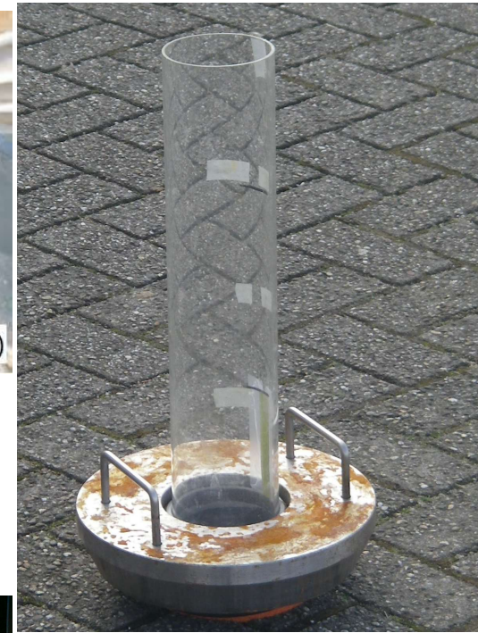
Modified Ring Infiltrometers used for Permeable Pavement Testing: a) DRIT (Fassman & Blackbourn, 2010); b) Square, Double Ring (Lucke & Beecham, 2011); c) Single Ring Surface Inundation Test (Bean et al., 2004) . Right: permeable stone measurements
