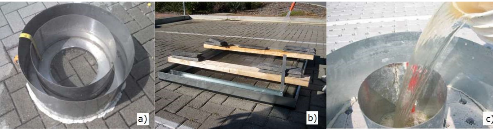
Modified Ring Infiltrometers used for Permeable Pavement Testing: a) DRIT (Fassman & Blackbourn, 2010); b) Square, Double Ring (Lucke & Beecham, 2011); c) Single Ring Surface Inundation Test (Bean et al., 2004) . Right: permeable stone measurements
